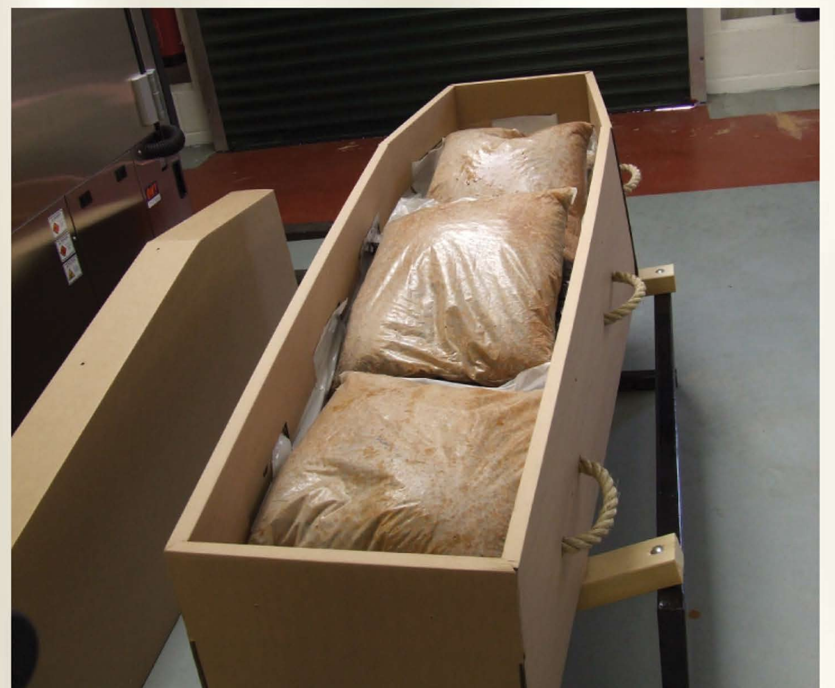
Picture taken (with lid removed) throughout over Load Test. Load of 49st, 8.9lb (315.2kg).
