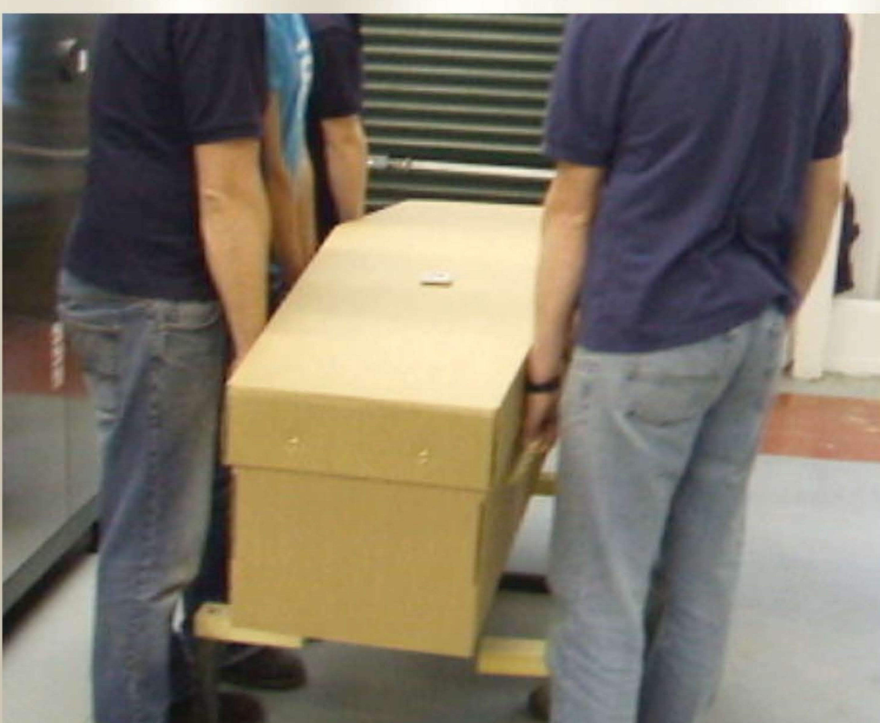
Coffin not affected by the 150kg load and lift.
