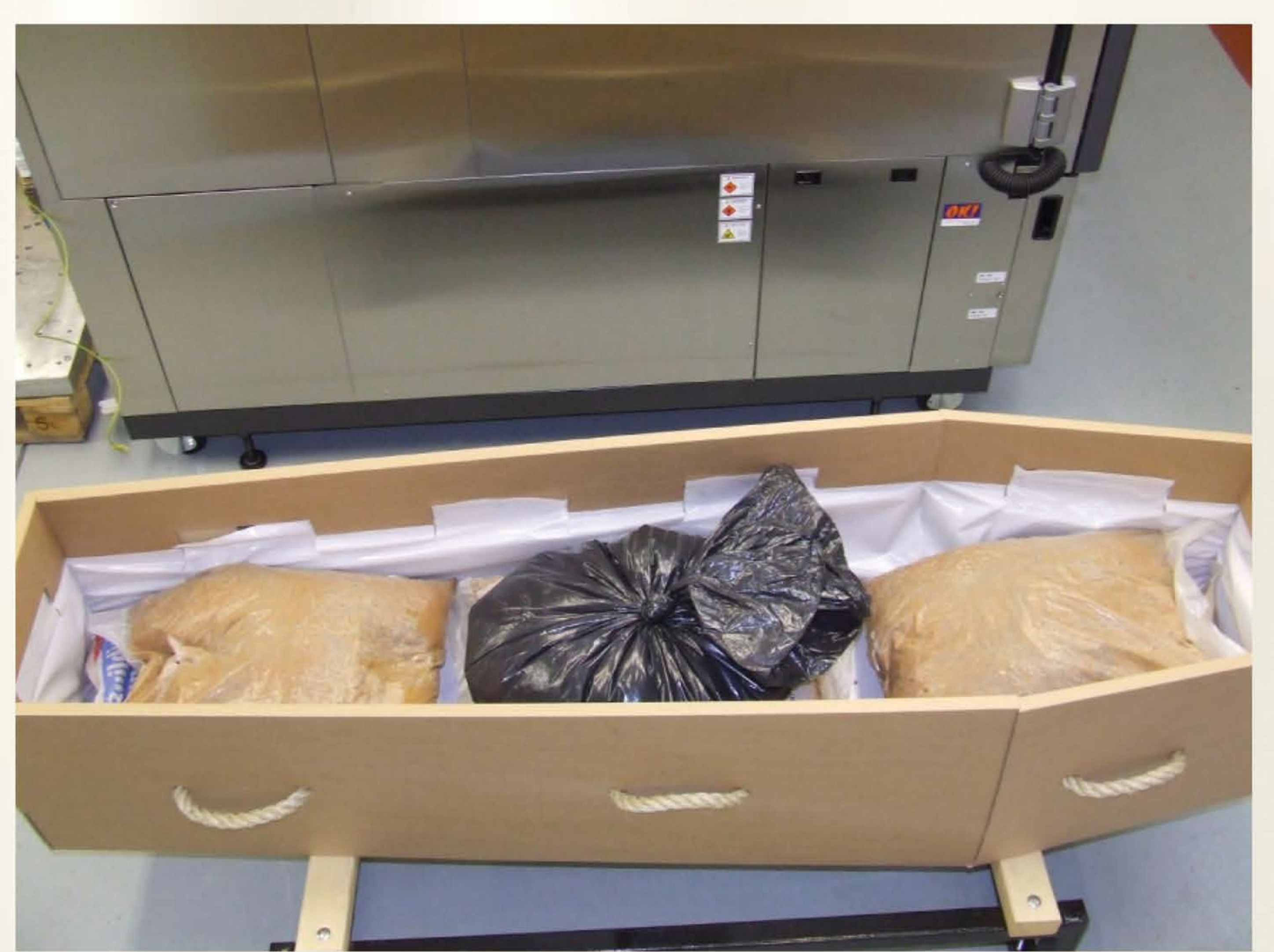
Coffin placed on stand with 150kg loaded. Coffin was not affected by the 150kg load.
